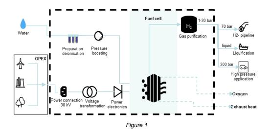
For example, the plant components required for hydrogen storage, transport and transformation from high to medium voltage are not included within these (battery) limits and are therefore not included in the calculation of Capex.<sup>5</sup>
